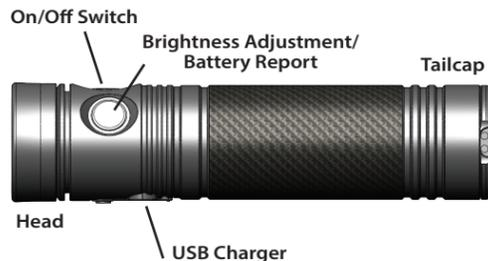
**WARNING** Included li-ion battery do not have any built-in battery protection. Take extreme care while handling them. Serious damage can occur if the battery is shorted, over-discharge/charged.
